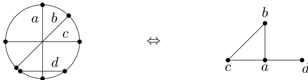
Figure 2.3: A circle with four chords and the corresponding circle graph
